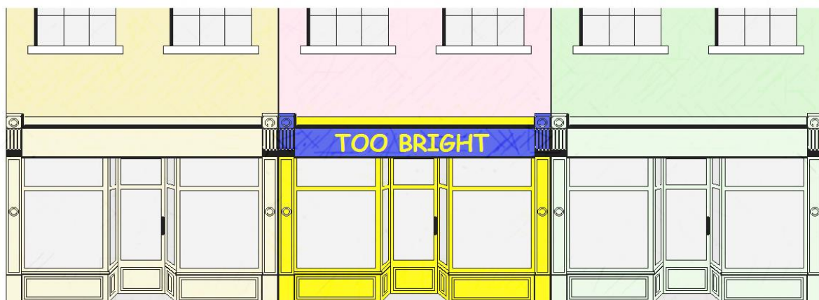
Figure 4: Example where middle shopfront is out of keeping with the wider terrace, and detracts from the character and appearance due to unsympathetic colour choice.
