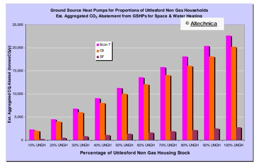
Figure 4-13: Estimated Potential Aggregated CO<sub>2</sub> abatement from switching space & water heating of 10 to 100% of <u>non-gas</u> households in Uttlesford to GSHPs powered by mains electricity.
