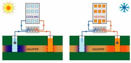
Summer: cooling of office buildings/industrial processes Winter: heating of office buildings/industrial processes Figure 4-39: Diagram of Aquifer Thermal Energy Storage system (Source IF Tech Ltd)
