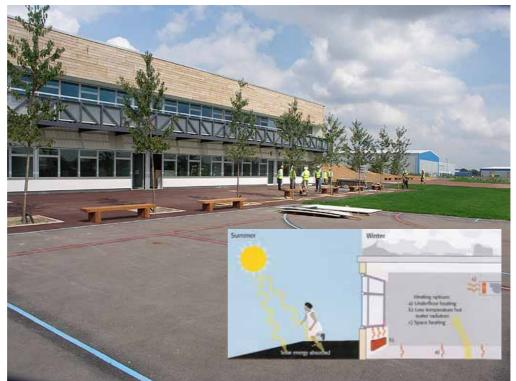
Figure 4-38: The ICAX IHT sandwich type systm for using a playground for solar-assisted ground coupled energy for heating a school in Hertfordshire. Source ICAX Ltd
