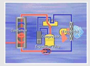
Figure 4-5: Diagram of a Compression type Heat Pump (Alliant)
