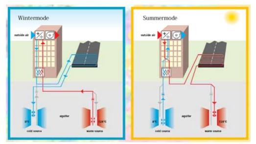
Figure 4-35: Diagram of the *Road Energy System* using roads for solar-assisted ground coupled energy. Source: Ooms
