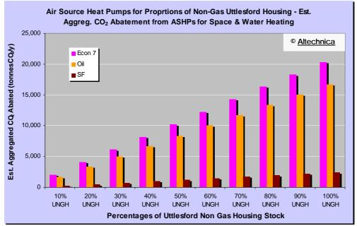
**Figure 4-32:** Estimated Potential Aggregated CO<sub>2</sub> abatement from switching space & water heating of 10 to 100% of non-gas households in Uttlesford to ASHPs powered by mains electricity.
