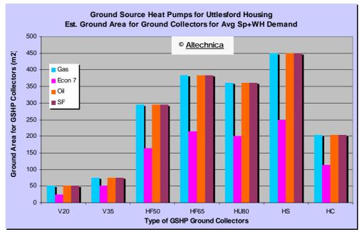
**Figure 4-16:** Ball Park Estimates of required ground area for vertical and horizontal GSHP Ground Collectors. V20 =  $20m/kW_{TH}$  vertical collector; V35 =  $35m/kW_{TH}$  vertical collector; HF50 =  $50m/kW_{TH}$  horizontal flat collector; HF65 =  $65m/kW_{TH}$  horizontal flat collector; HU80 =  $80m/kW_{TH}$  horizontal upright collector; HS = Horizontal upright 'Slinky'; HC = Horizontal compact collector.
