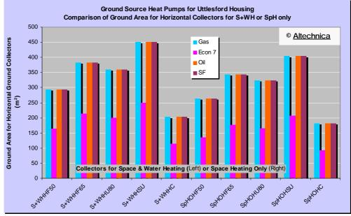
Figure 4-17: Ball Park Estimates of required ground area for horizontal GSHP Ground Collectors showing ground area requirements when providing the estimated average space and water heating (S+WH) needs (left) & when the GSHPs are sized to provide only the estimated space heating (SpH) demand.
