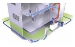
**Figure 4-4**: Example of a proprietary Earth Tube Ring. (Source Rehau)
