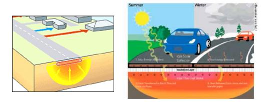
Figure 4-37: The ICAX IHT sandwich type systm for using roads for solar-assisted ground coupled energy. Source ICAX
