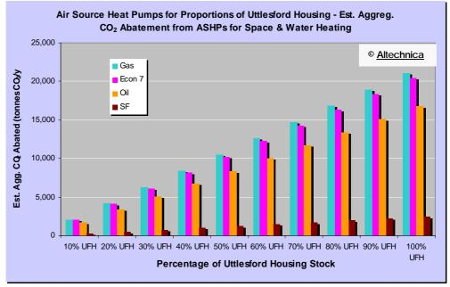
Figure 4-31: Estimated Potential Aggregated  $CO_2$  abatement from switching space & water heating of households in Uttlesford to ASHPs powered by mains electricity.
