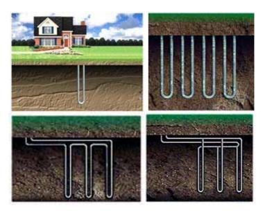
Figure 4-7: Vertical U-Tube Ground / Collector Heat Exchangers for Ground Source Heat Pump. Bottom Left: 'Series' collector, Bottom Right: 'Parallel' Collector. Note: vertical dimension shortened diagrammatically. (Alliant)
