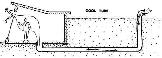
Figure 4-2: Earth Tube/Pipe operating as a Cool Tube for cooling incoming ventilation air. (Boyer etal. 1987)
