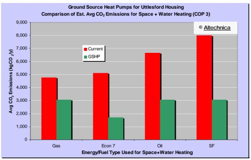
**Figure 4-10:** Comparison of Estimated Annual Average  $CO_2$  emissions to deliver estimated Annual Average Uttlesford Household Space & Water Heating Demands (according to energy/fuel type). Compares  $CO_2$  emitted from GSHPs (using mains electricity) with Current Energy/Fuel Type.
