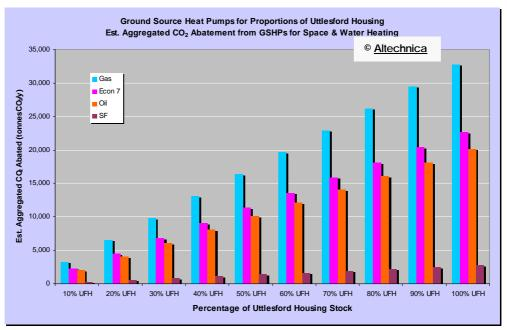
**Figure 4-12:** Estimated Potential Aggregated CO<sub>2</sub> abatement from switching space & water heating of households in Uttlesford to GSHPs powered by mains electricity.
