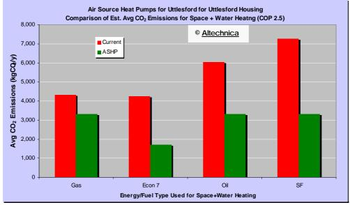
**Figure 4-29:** Comparison of Estimated Annual Average  $CO_2$  emissions to deliver estimated Annual Average Uttlesford Household Space & Water Heating Demands (according to energy/fuel type offset). Compares  $CO_2$  emitted from ASHPs (using mains electricity) with Current Energy/Fuel Type.
