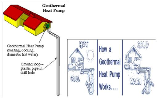
Figure 4-8: The ground source heat pump extracts useful ambient heat from below ground.
