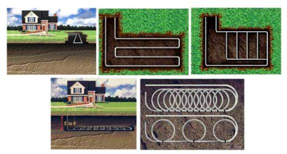
Figure 4-6: Horizontal Ground Collector Heat Exchangers for Ground Source Heat Pump. Top Middle: Plan view of a 'Series' Collector, Top Right: Plan View of 'Parallel' Collector, Bottom 'Slinky' Coil Collector. (Alliant)
