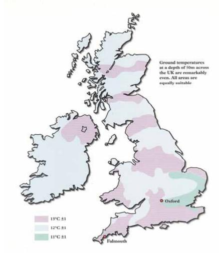
Figure 4-1: Map of ground temperatures around the UK at a depth of 50 m. (Source: Geoscience)
