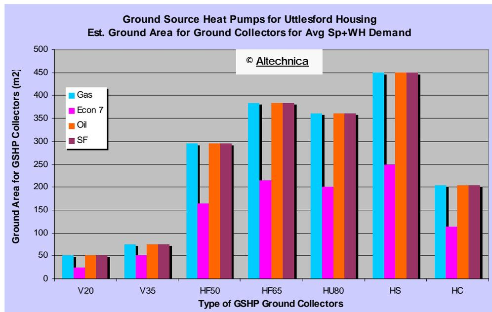
**Figure 4-16:** Ball Park Estimates of required ground area for vertical and horizontal GSHP Ground Collectors. V20 = 20m/kW<sub>TH</sub> vertical collector; V35 = 35m/kW<sub>TH</sub> vertical collector; HF50 = 50m/kW<sub>TH</sub> horizontal flat collector; HF65 = 65m/kW<sub>TH</sub> horizontal flat collector; HU80 = 80m/kW<sub>TH</sub> horizontal upright collector; HS = Horizontal upright 'Slinky'; HC = Horizontal compact collector.
