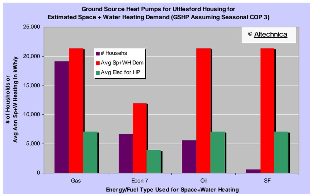
**Figure 4-9:** Estimated Annual Average Uttlesford Household Space & Water Heating Demand, Numbers of Households & Annual Average GSHP Electricity according to Current Energy/Fuel Type (e.g. gas, Economy 7 electricity, oil or solid fuel).
