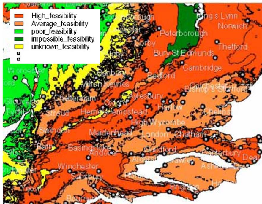
Figure 4-40: Aquifer Thermal Energy Storage (ATES) Map Including Uttlesford (Source IF Tech Ltd)
