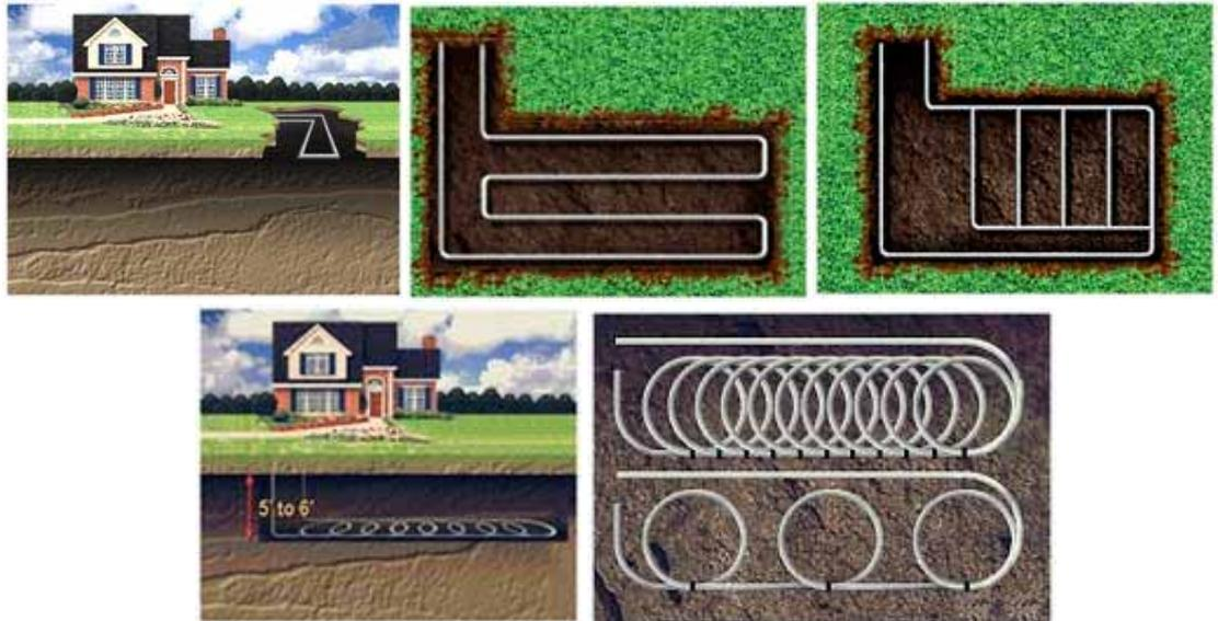
**Figure 4-6:** Horizontal Ground Collector Heat Exchangers for Ground Source Heat Pump. Top Middle: Plan view of a 'Series' Collector, Top Right: Plan View of 'Parallel' Collector, Bottom 'Slinky' Coil Collector. (Alliant)
