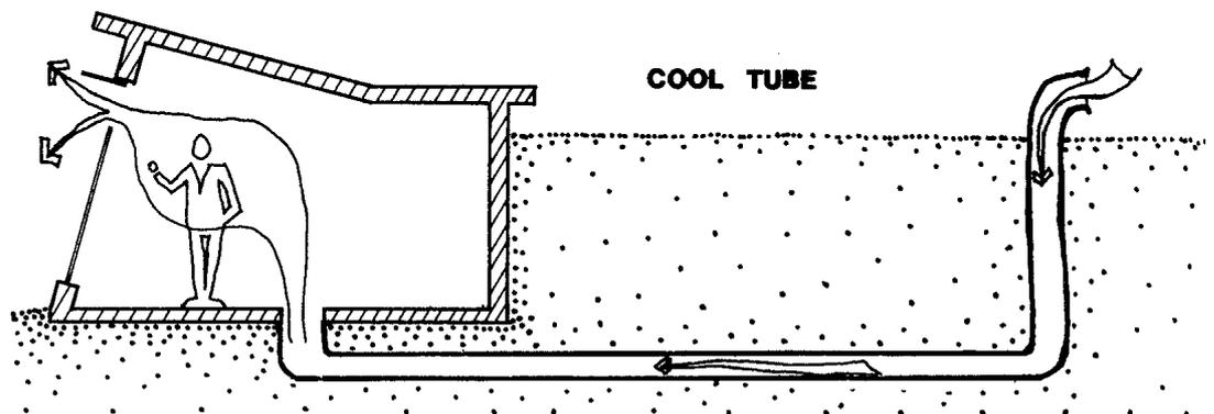
**Figure 4-2:** Earth Tube/Pipe operating as a Cool Tube for cooling incoming ventilation air. (Boyer et al. 1987)
