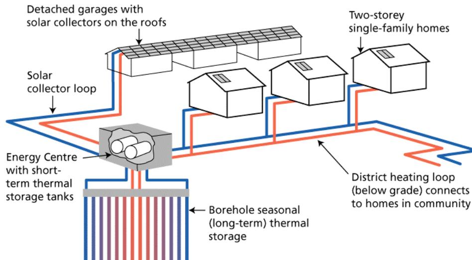
**Figure 4-41:** BTES used for inter-seasonal storage for 52 homes in Drakes Landing Solar Community in Canada (Source Drakes Landing Community)
