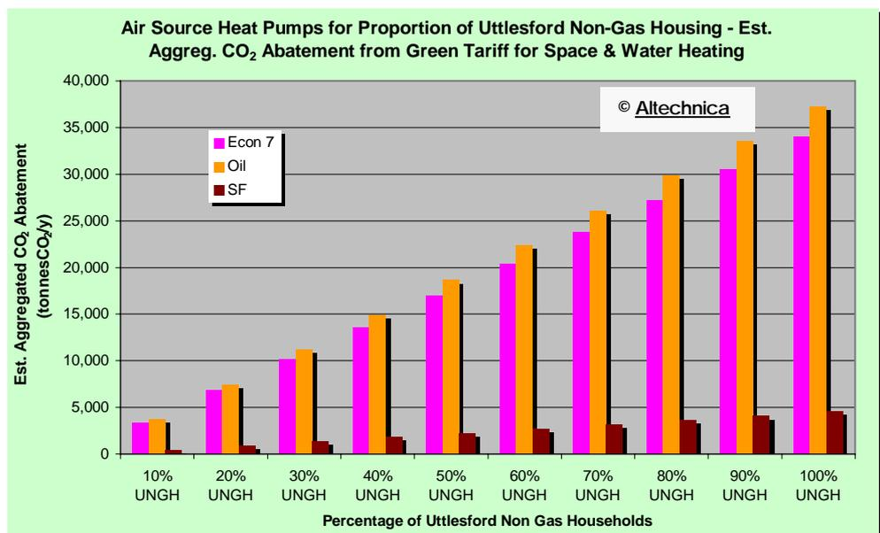
Figure 4-34: Ball park estimates of aggregated CO<sub>2</sub> emissions abatement from CO<sub>2</sub>-free Green Tariff Powered ASHPs for space and water heating for 10 to 100% of Uttlesford Non Gas households. Seasonal COP of 3.
