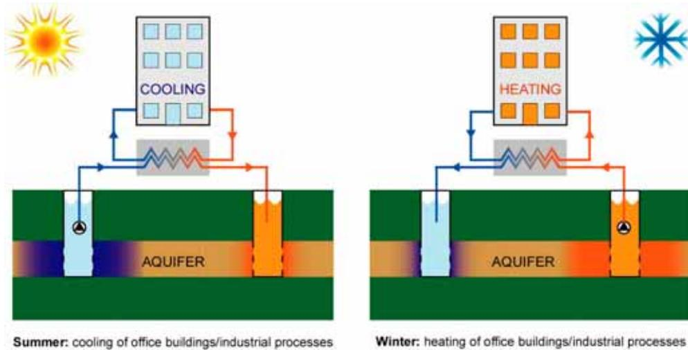
Figure 4-39: Diagram of Aquifer Thermal Energy Storage system (Source IF Tech Ltd)
