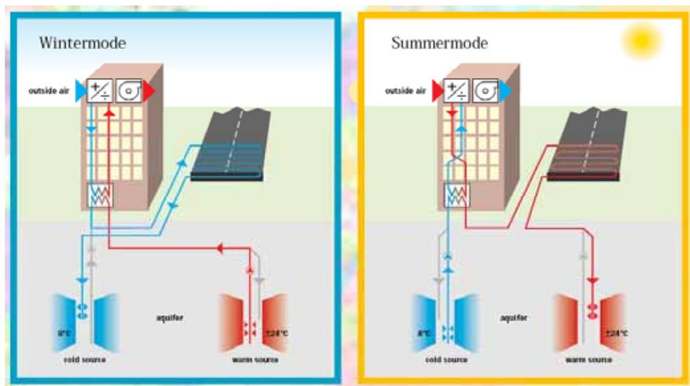
**Figure 4-35:** Diagram of the *Road Energy System* using roads for solar-assisted ground coupled energy. Source: Ooms
