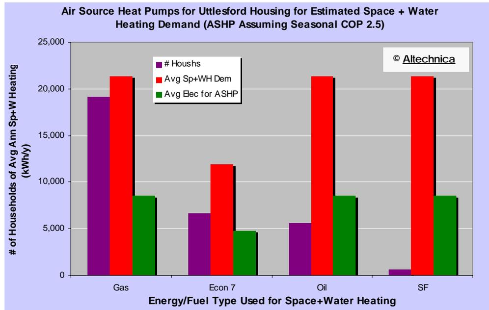
**Figure 4-19:** Estimated Annual Average Uttlesford Household Space & Water Heating Demand, Numbers of Households/energy type & Annual Average ASHP Electricity according to Current Energy/Fuel Type offset (e.g. gas, Economy 7 electricity, oil or solid fuel).
