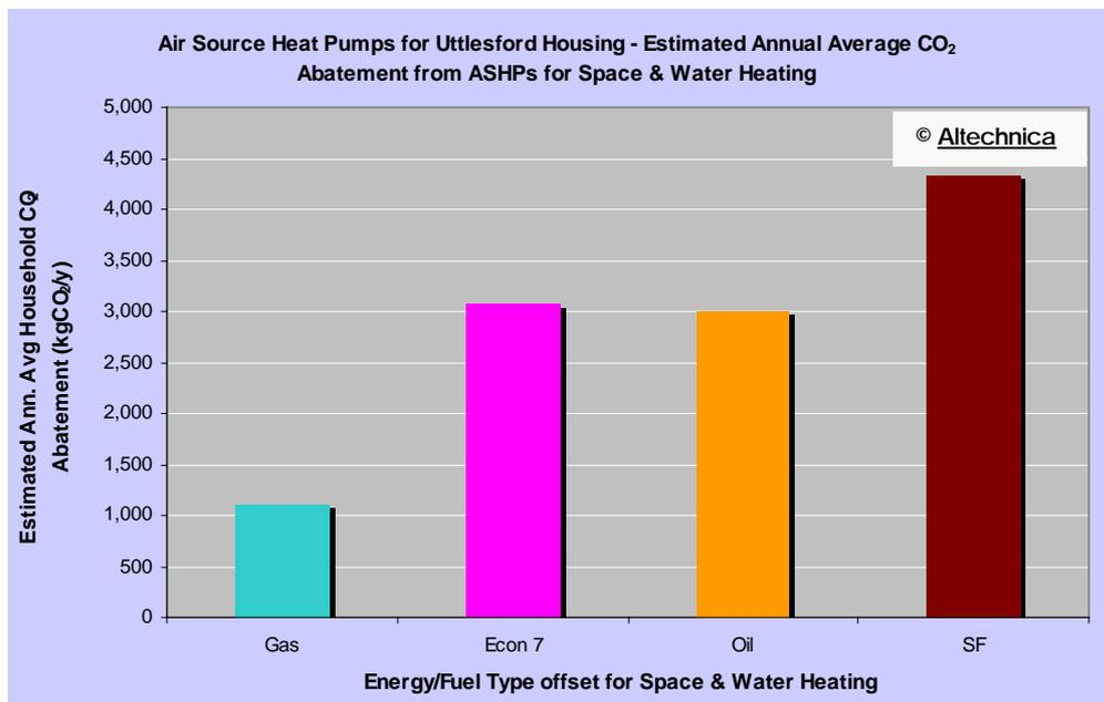
**Figure 4-30:** Estimated annual average CO<sub>2</sub> abatement/household from ASHPs displacing space & water heating.
