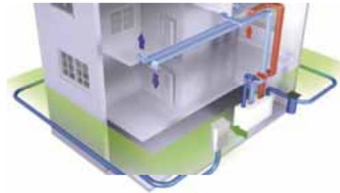
**Figure 4-4:** Example of a proprietary Earth Tube Ring. (Source Rehau)
