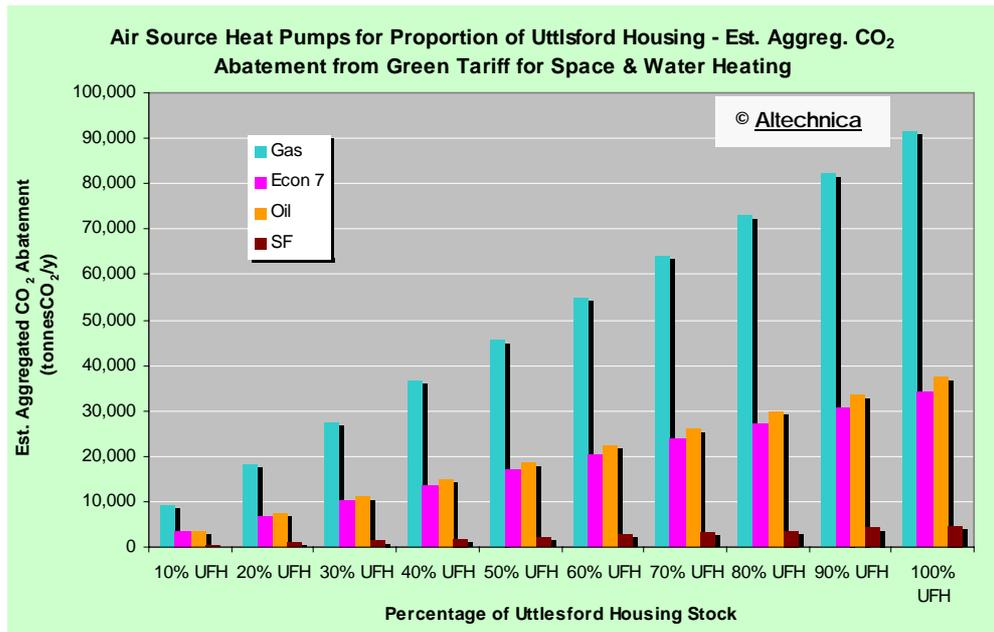
Figure 4-33: Ball park estimates of aggregated CO<sub>2</sub> emissions abatement from CO<sub>2</sub>-free Green Tariff Powered ASHPs for household space and water heating for 10 to 100% of Uttlesford households. Seasonal COP of 2.5.
