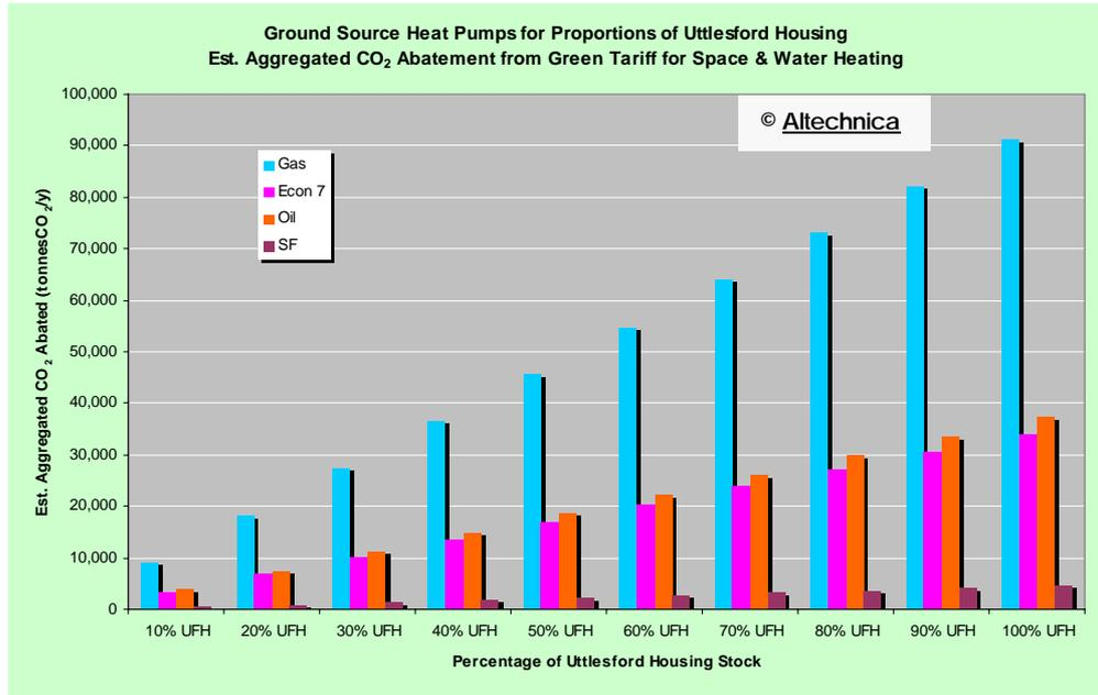
Figure 4-14: Ball park estimates of aggregated CO<sub>2</sub> emissions abatement from CO<sub>2</sub>-free Green Tariff powered GSHPs for household space and water heating for 10 to 100% of Uttlesford households. Seasonal COP of 3.
