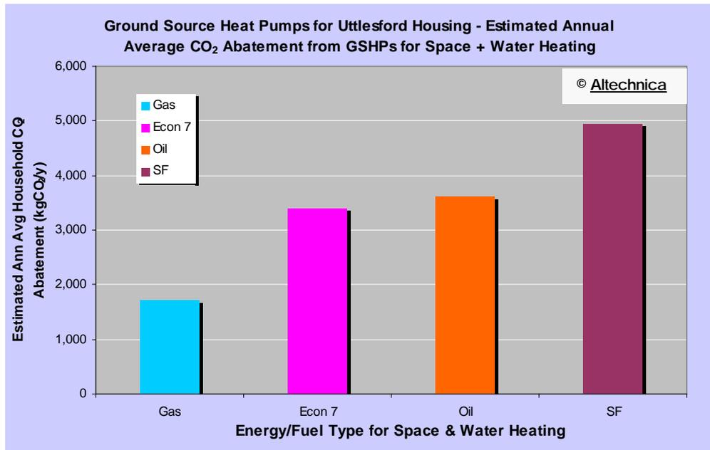
Figure 4-11: Estimated Annual average CO<sub>2</sub> abatement/household by GSHPs displacing space & water heating.
