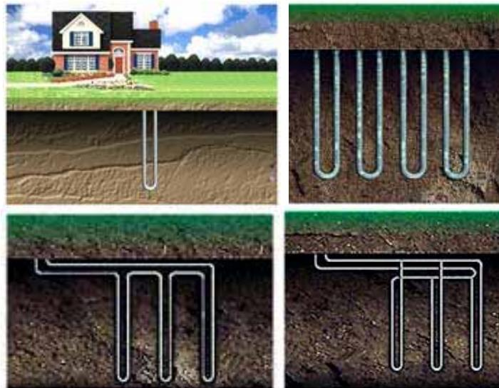
**Figure 4-7:** Vertical U-Tube Ground / Collector Heat Exchangers for Ground Source Heat Pump. Bottom Left: 'Series' collector, Bottom Right: 'Parallel' Collector. Note: vertical dimension shortened diagrammatically. (Alliant)
