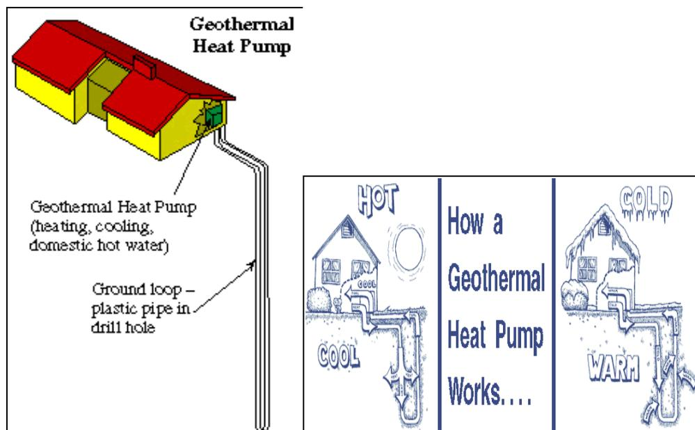
**Figure 4-8:** The ground source heat pump extracts useful ambient heat from below ground.
