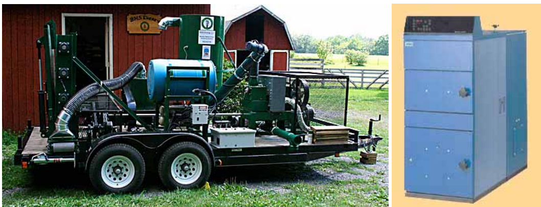
Figure 5-15 (a) Prototype mobile straw & grass pellet mill (left) (Source BHS). (b) Grain boiler (right) (Baxi).
