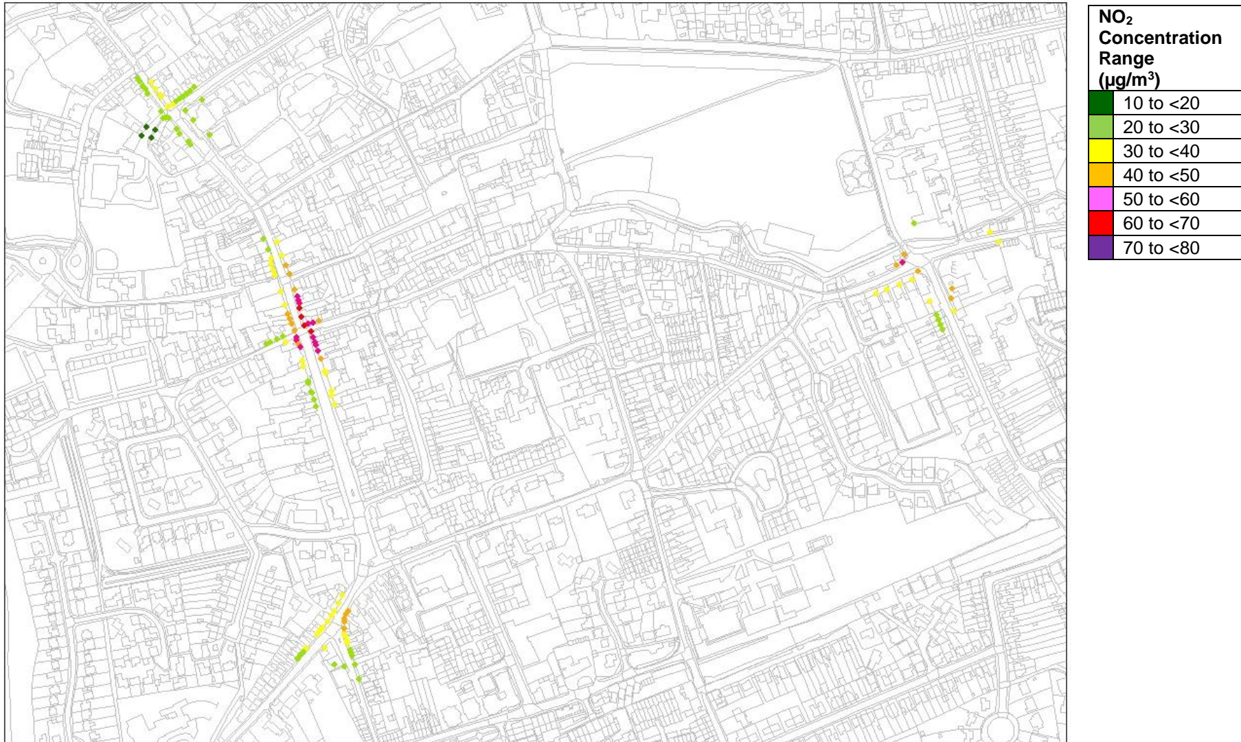
Figure 6-H: 2018 Full Scheme Scenario – Modelled Annual Mean NO 2 Concentrations (based on the LTT Methodology)
