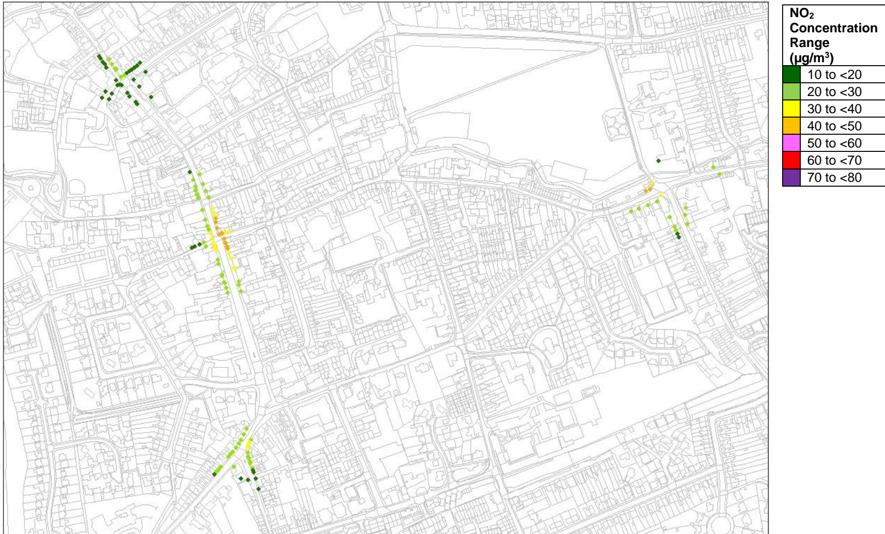
Figure 6-E: 2018 Do Minimum Scenario – Modelled Annual Mean NO 2 Concentrations (based on the LAQM TG09 Methodology)
