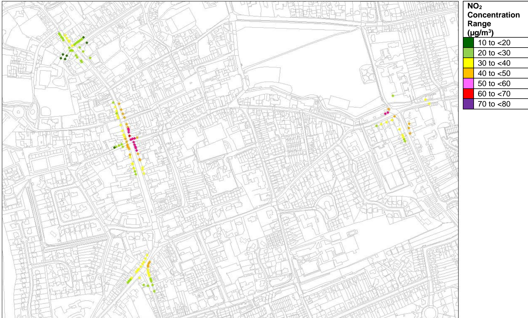
Figure 6-L: 2026 Do Minimum Scenario – Modelled Annual Mean NO 2 Concentrations (based on the LTT Methodology)
