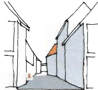
Drop in height compensated by rise in height on opposite side of space at A
