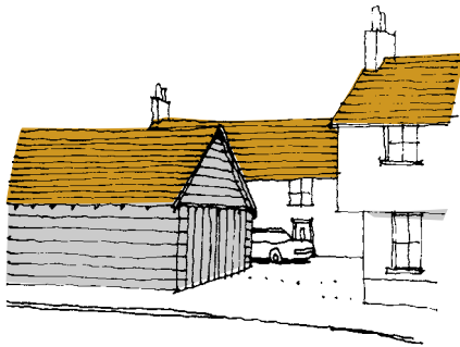
Double garages placed back to back to form barn-like structure
