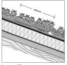
Image 107 Green roof section Courtesy of Bauder Ltd.
