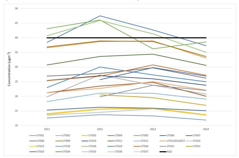
Analysis of UK continuous  $NO_2$  monitoring data has shown that it is unlikely that the hourly mean  $NO_2$  objective, of 18 hourly means over 200  $\mu$ gm<sup>-3</sup>, would be exceeded where the annual mean objective is below  $60\mu$ gm<sup>-3</sup> (Defra, 2009). All sites diffusion tube sites in Uttlesford have measured concentrations below the  $60\mu$ gm<sup>-3</sup>, therefore, the  $NO_2$  hourly mean AQS objective is expected to be met at all relevant locations.
