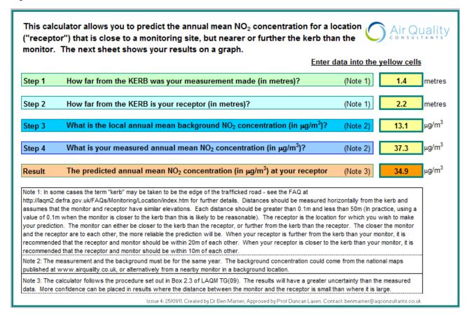
Figure B4 UT028 diffusion Tube NO<sub>2</sub> fall off with distance calculations
