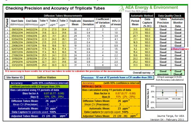
A local bias adjustment factor was calculated of 0.87 for all automatic and diffusion tube data, as shown in Figure B2.
