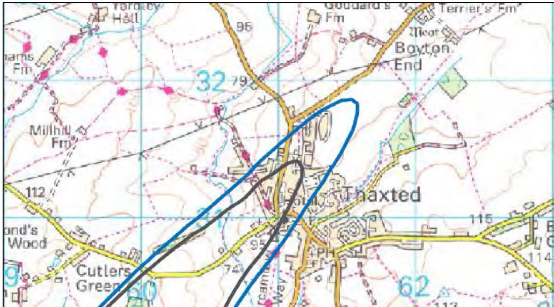
Figure 7.9: Extent of 2028 54 dB L_{Aeq,8h} summer night contour over Thaxted: DC = blue, DM = black
