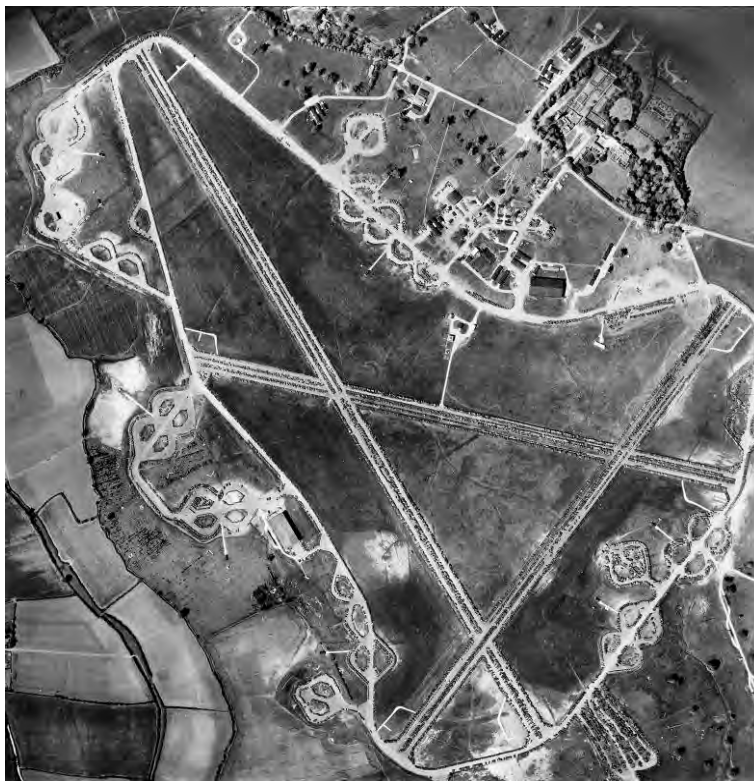
Fig 11: Aerial photograph of RAF Great Dunmow aerodrome in May 1948. The runways, perimeter track and hard standings are being used for storage of now redundant military vehicles
