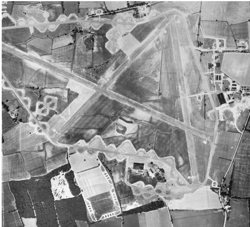
Fig. 8: Aerial photograph of RAF Great Saling / Andrewsfield in August 1949. Although longer an operational aerodrome the runways, perimeter track, hard standings, hangers, buildings and munitions dumps are still intact.
