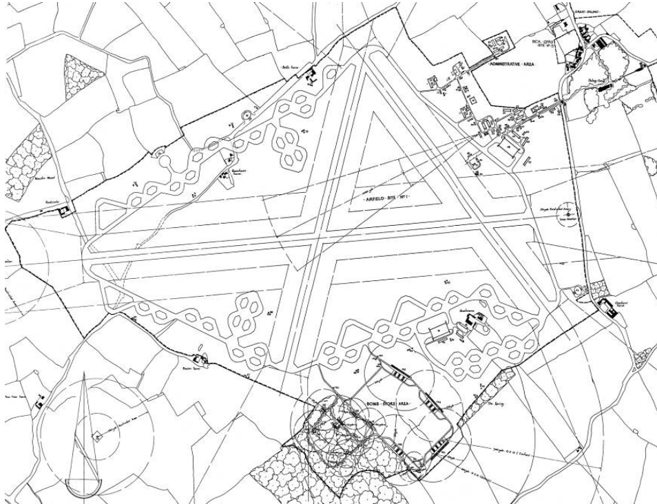
Fig. 6: Plan of RAF Great Saling / Andrewsfield aerodrome in 1943 showing location of the three runways, perimeter track with dispersal hard standings and munitions dump. Great Saling is located top right of the plan.
